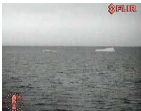
These bergy bits deflect radar signals away from the antennae, but they show up clearly on a thermal image.
