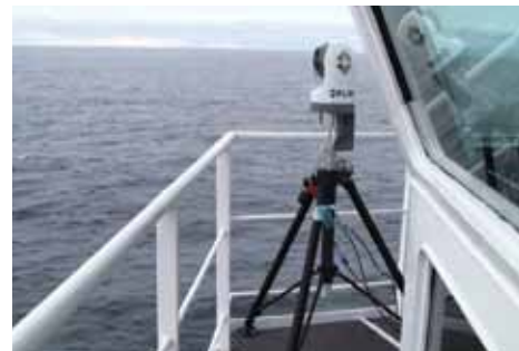
For the test two models of the M-Series were mounted on a tripod next to the bridge of an ice strengthened vessel that traverses the Arctic waters of Greenland.
